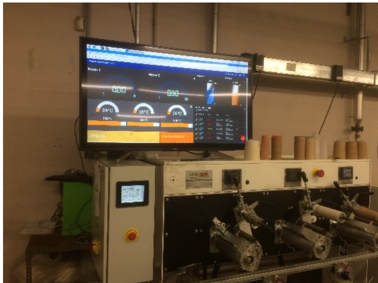
Example of a retrofitted machine using Thingsboard IoT platform
